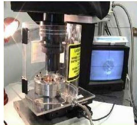
SONY camera (through a National Instruments PCI-1408) and numerous vacuum valves (National Instruments PCI- 6503). Two PCs are used to control the system – one in the light-tight room directly controlling the system, and a second in the technician's room for process definition and control, and system monitoring.
