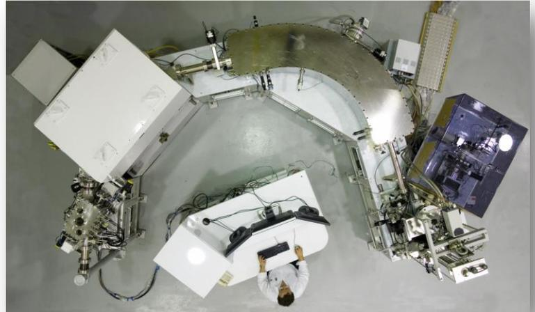
The *SHRIMP* was designed specifically to operate in a teaching environment, where relatively inexperienced users have access to the instrument, so it was vital to ensure that unnecessary complexity was avoided, systems and electronics were robust and operation as straightforward as possible. Also, the design team recognised the need for easy access during maintenance and to make routine operations as simple as possible.
